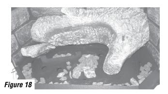
Place the rockwool (F) over the gas ports and in between the embers along the front of the firebox. The rockwool can be placed over gas ports but do not cover the secondary air holes (see *Burner Pan Diagram*, *Page 10*).
